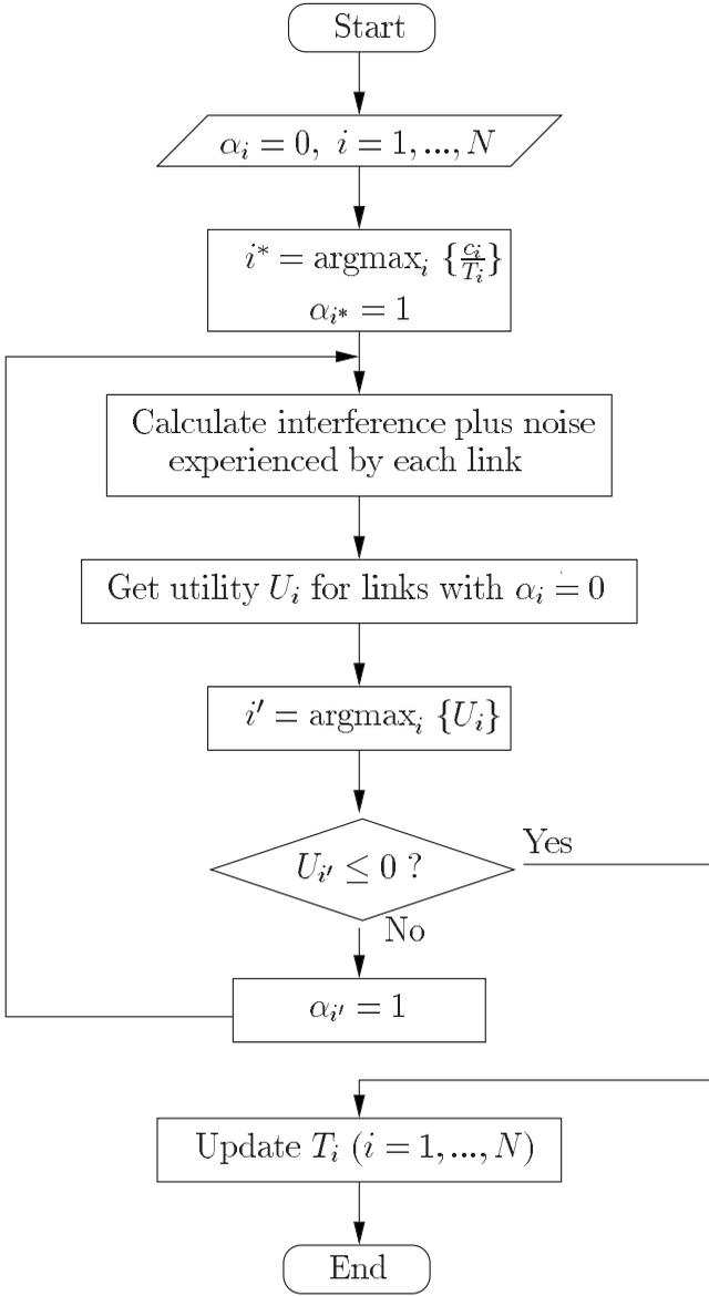
Fig. 3. The scheduling procedure (in a packet slot) of water-adding scheme with fairness adaptation.
