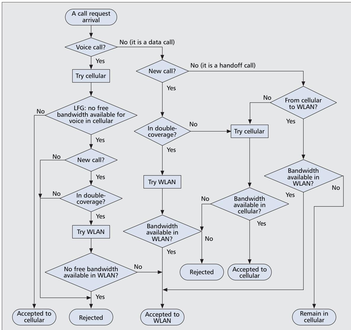
■ Figure 3. Call admission procedure for cellular/WLAN interworking.
