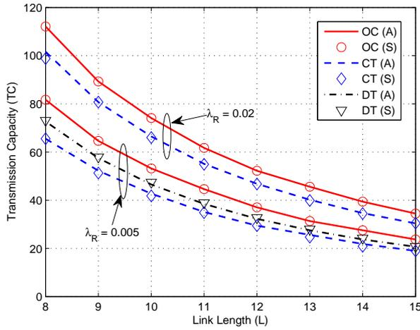
**Fig. 7** Transmission capacity in links/km<sup>2</sup> versus link length for  $\lambda_R = 0.005$  nodes/m<sup>2</sup> and  $\lambda_R = 0.02$  nodes/m<sup>2</sup> when  $r_C = 4$  m and  $\kappa = 0.5$
