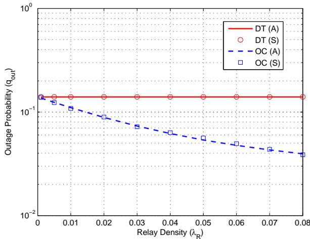
**Fig. 4** Outage probability versus relay density (in nodes/m<sup>2</sup>) when  $\lambda_S = 0.0001$  nodes/m<sup>2</sup>,  $r_C = 4$  m,  $\kappa = 0.5$ , and  $L = 12$  m
