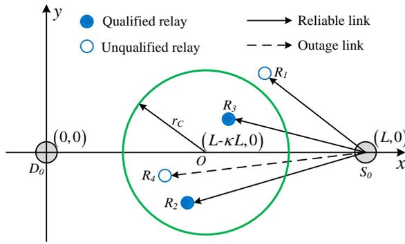
**Fig. 1** An illustration of the constrained relay selection region centered at  $O$  with radius  $r_C$  for the target source-destination pair under the 2D Cartesian coordinate system. Only the relays within the constrained relay selection region (e.g.,  $R_2$ ,  $R_3$ , and  $R_4$ ) that successfully receive the packet from the source (e.g.,  $R_2$  and  $R_3$ ) are qualified relays (e.g.,  $R_2$  and  $R_3$ )
