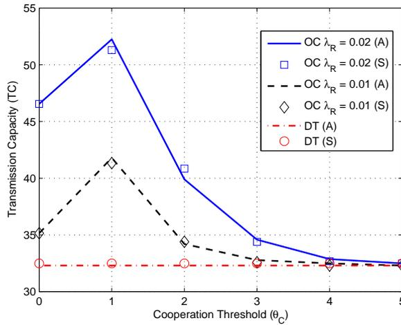
**Fig. 5** Transmission capacity in links/km<sup>2</sup> versus cooperation threshold for  $\lambda_R = 0.01$  nodes/m<sup>2</sup> and  $\lambda_R = 0.02$  nodes/m<sup>2</sup> when  $r_C = 4$  m,  $\kappa = 0.5$ , and  $L = 12$  m
