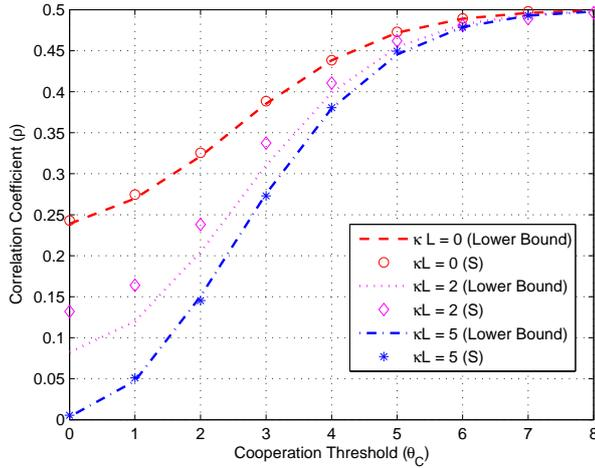
**Fig. 3** Correlation coefficient of interference power  $I_{D_0:1}(\Phi_D, \Phi_C)$  and  $I_{D_0:2}(\Phi_D, \Phi_F)$  versus cooperation threshold  $\theta_C$  and distance between a source and the center of a relay selection region  $\kappa L$  when  $\lambda_S = 0.001$  nodes/m<sup>2</sup>,  $\lambda_R = 0.2$  nodes/m<sup>2</sup>,  $r_C = 2$  m, and  $L = 12$  m
