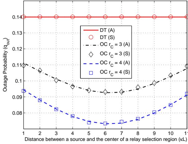
**Fig. 6** Outage probabilities versus distance between a source and the center of a relay selection region for  $r_C = 3$  m and  $r_C = 4$  m when  $\lambda_S = 0.0001$  nodes/m<sup>2</sup>,  $\lambda_R = 0.03$  nodes/m<sup>2</sup>, and  $L = 12$  m
