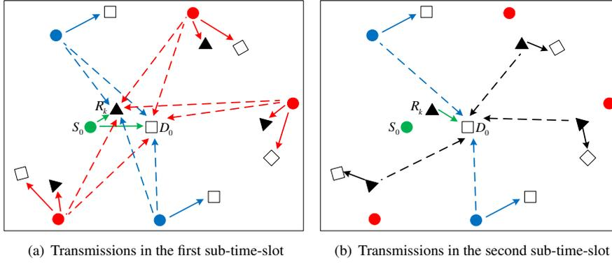
**Fig. 2** An illustration of the interference power, originating from both the direct and cooperative links over the network, observed by relay  $R_k$  and destination  $D_0$  in the first and second sub-time-slots. Each circle, triangle, and square represent a source, selected relay, and destination, respectively. The solid and dashed lines represent the transmitted signal and interference, respectively
