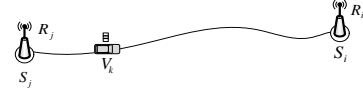
Fig. 5. Packet propagation from one social spot S_j to its neighboring social spot S_i through vehicle V_k .
