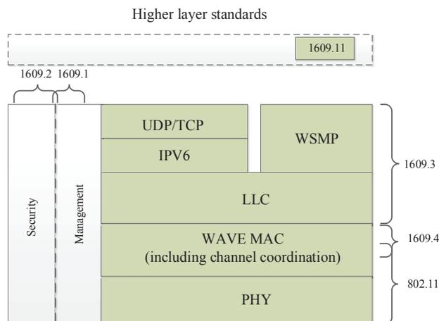
Fig. 4. Protocol stack of WAVE.
