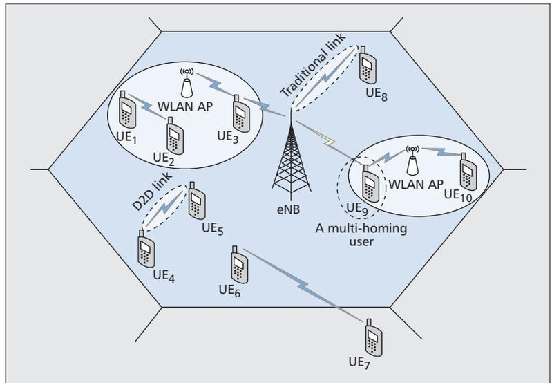
**Figure 1.** Underlying cellular/WLAN converged D2D communication network.
